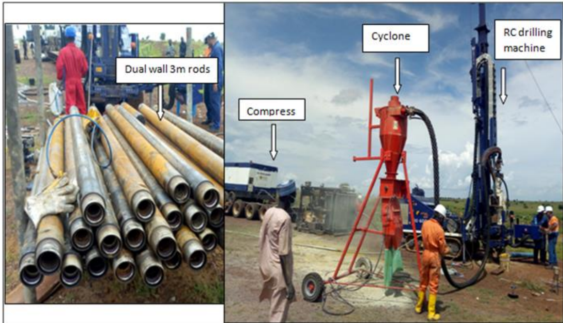
RC Drilling for phosphate resource within the Sokoto Basin using the Multipurpose Comacchio Geo 602 Explorer complete with Riffle Splitter
