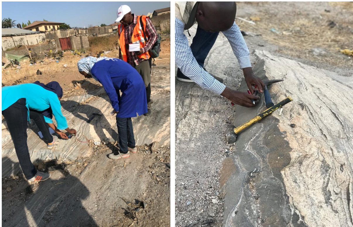
Taking the strike of foliation on the kabala gneiss at kabala costain, kaduna
