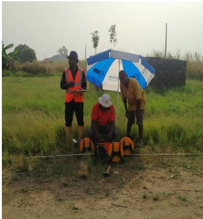
Vertical Electrical Sounding (VES) measurement to determine bore hole location
