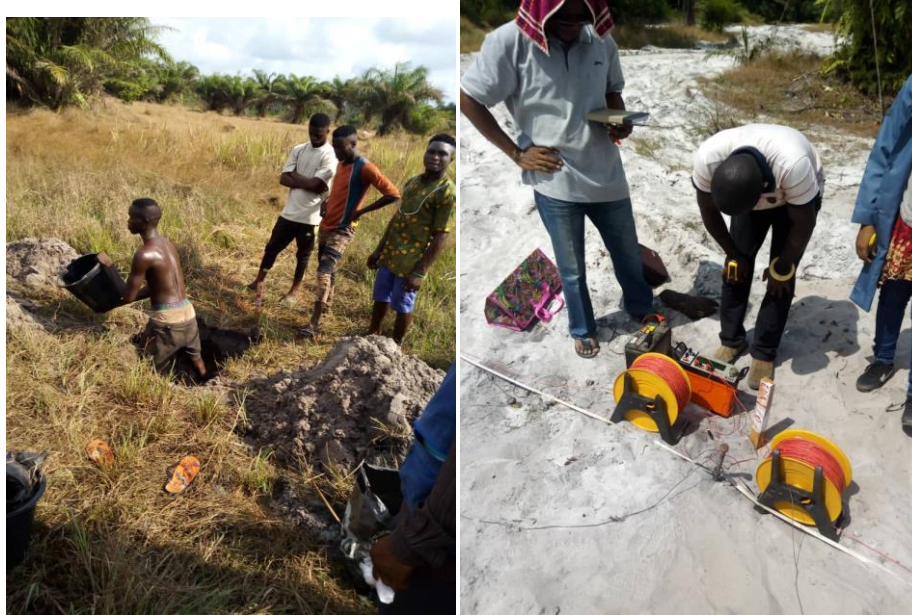
Pitting and Electrical Resistivity works at Igbokoda Silica Sand site
