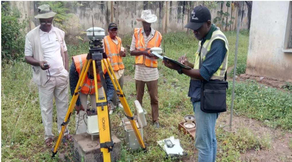
NGSA Geophysicist acquiring Gravity data for structural mapping and industrial mineral exploration (Kaolin, talc and marble) along Ilorin-Share Road
