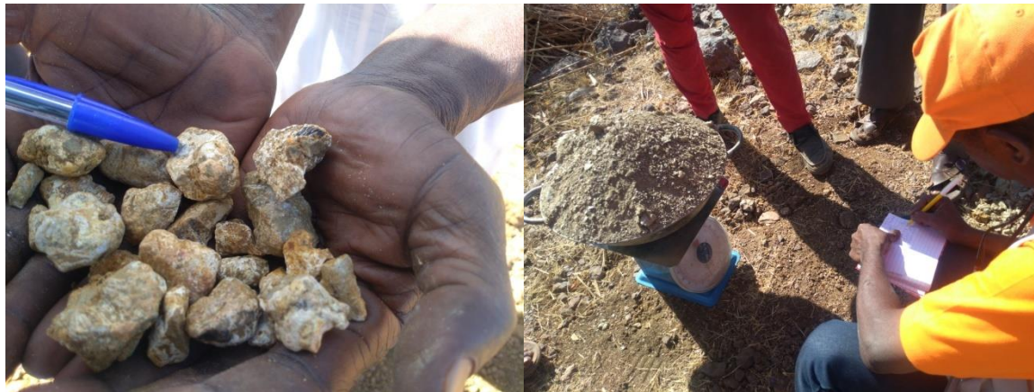
Phosphatic Nodules from a pit at Salame Recording first head pan of Shale with Phosphate nodule at Balakuzu area
