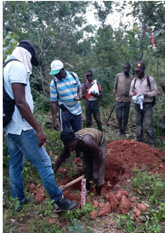
Measurement of magnetic susceptibility and pitting at Libele-Nasko
