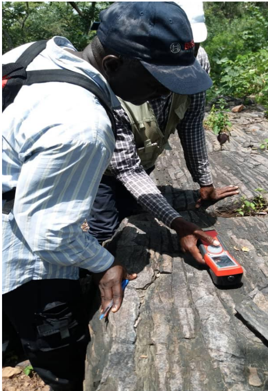
Measurement of magnetic susceptibility and pitting at Libele-Nasko
